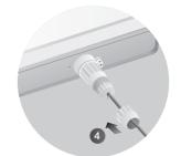
Note: To ensure waterproofing, choose the proper seal according to the type and diameter of the Ethernet cable.
